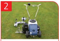
The BeamRider is then positioned close to the laser.
