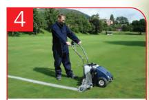
Once the receiver is locked onto the beam, turn on the spray marker and walk.
